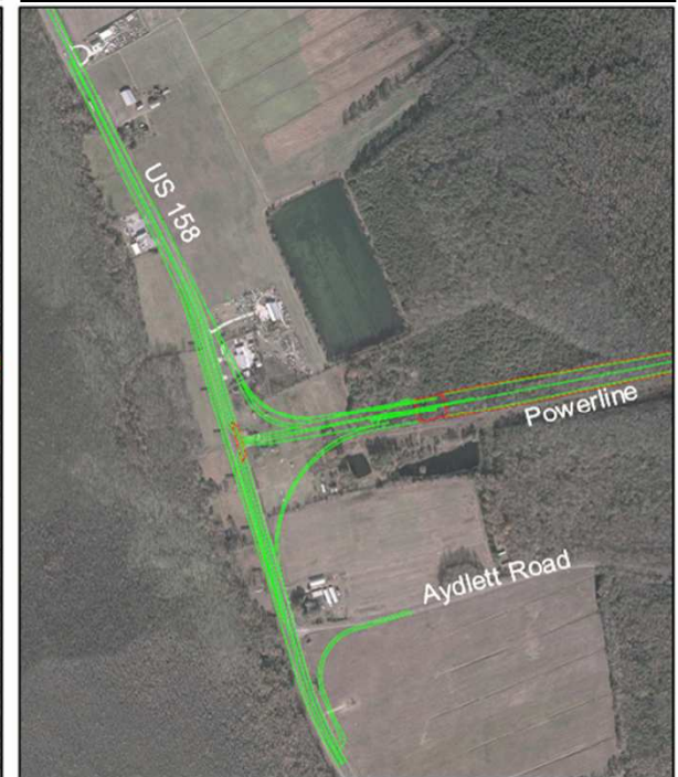
Partial Interchange/Intersection Design
