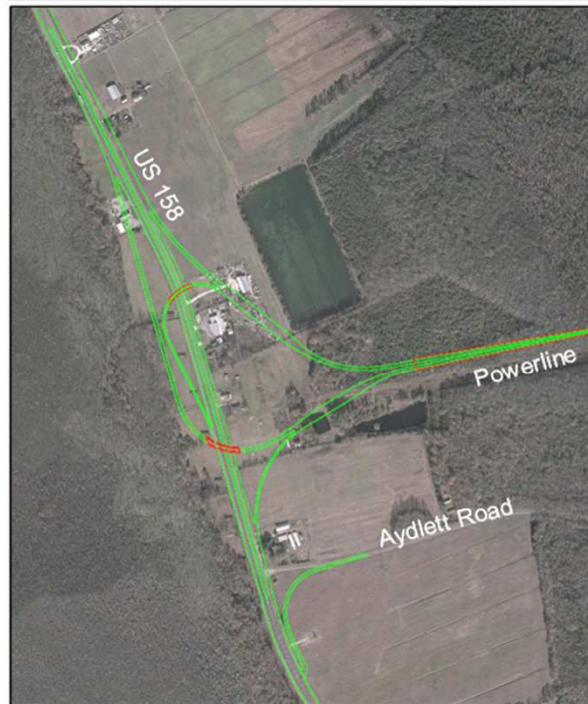
Compressed Y Interchange Design
